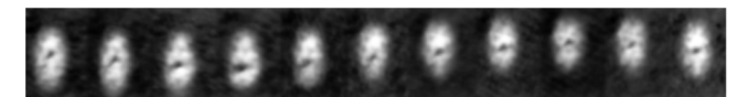
FIG. 3. Drag force on a Bose-Einstein condensate, derived as an asymmetry in the density profile (top). Beyond 4 mm/s the signal saturated due to the formation of a high-density bow wave, introducing nonlinearity into the phase contrast signal for phase shifts exceeding \pi . The bars represent statistical errors. Scanning the laser at the axial trapping frequency, corresponding to a stirring velocity of 1.5 mm/s for an amplitude of 37 \mu\text{m} , shows synchronous oscillations of the condensate (bottom) and reduced heating.
